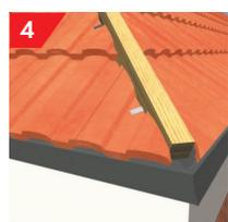
Commence tiling as normal, cutting tiles neatly along the line of the hip batten, making sure no cut tile is more than 30mm from the hip batten. Small tile cuts are secured using the fixing clips provided. The teeth of the clip are inserted into the cut edge of the tile, and the wire is nailed to the tiling batten or hip batten.
