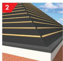
Hip batten supports, made up from 2 x 25mm thick tiling battens, are screwed to the hip rafter in between the tiling batten spaces. Hip batten supports need to be fixed at the eaves and apex and then spaced intermediately between the batten spaces, along the line of the hip rafter.
