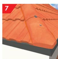
A block end hip tile is recommended at the eaves and should be mechanically fixed using 100mm screw and washer provided. Insert hip seals in between hip tiles and fix using the screw, washer and clamping plate provided, ensuring a minimum 15mm penetration into the hip batten. If the KR5000 or KR5100 kits are being used the ends of the ridge seals may be trimmed to suit the hip tile profile if required. Continue this process up to the apex.
