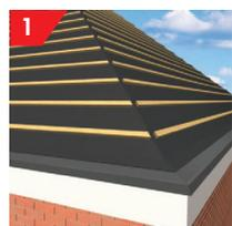
The roof underlay is laid in the normal way, making sure the tiling battens are secured directly onto the hip rafter or to noggins fixed to the side of the hip rafter in between the jack rafters. (This needs to be carried out before the underlay is laid).
